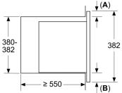
A: Overhang at top: 1 mm B: Overhang at bottom: 1 mm
