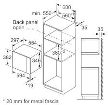
measurements in mm
