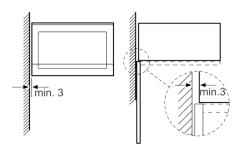
Measurements in mm
