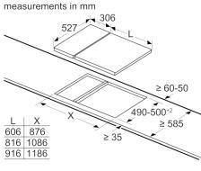
When installing a Domino unit right next to a hob, an assembly kit (HEZ394301) is required.
