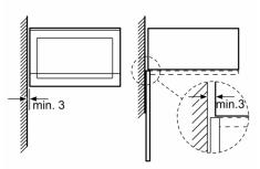
Measurements in mm
