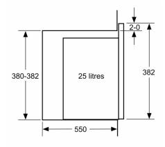
measurements in mm
