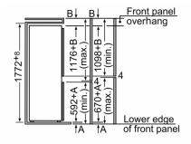
The specified unit door dimensions are valid for a door gap of 4 mm. If a different gap width is used (max. 14 mm), the dimensions must be adjusted.
